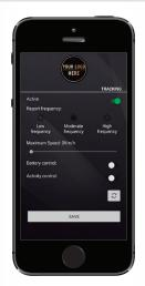
Each app can be preset to report its location to the server according to a time-distance routine calculation, setting these 2 parameters for each unity however it's convenient. administrators of a group can preset it on and off, as well as modify the units of time-distance of each member. The location report will run with the app on the background, even if the user is not using it.
